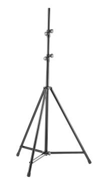
Extending to over 4 m, this lighting stand is for professional use. The new zinc die-cast clamps and the larger steel leg tubing give this top of the range stand more stability. The infinitely variable non-marring height adjustment can be reinforced with two safety rings. A variety of crossbars may be attached using the M10 thread adaptor.
