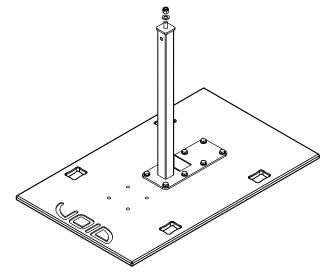
Figure 7.7: Stasys Xair/X V2 or Stasys 218 mounting board with bracket
