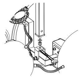
Figure 7.22: Air Motion ceiling mount detail
