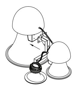
Figure 7.3: M8 LF driver removal
