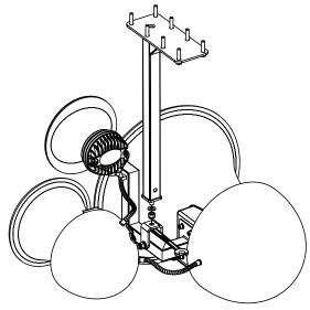
Figure 7.21: Air Motion ceiling mount
