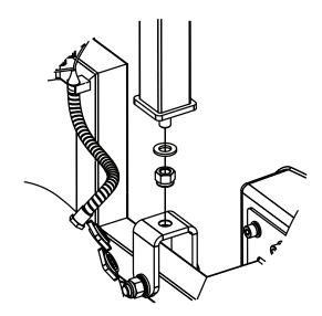
Figure 7.29: Air Motion truss mount detail
