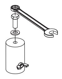
Figure 7.37: Pole mount bracket removal
