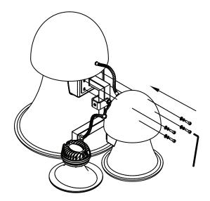
Figure 7.6: M8 socket cap reattaching
