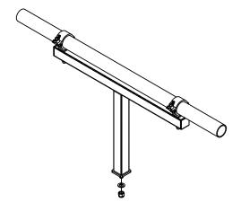
Figure 7.27: Attaching the truss bracket
