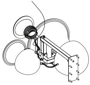
Figure 7.18: Safety wire attachment
