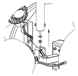
Figure 7.33: Attaching the Air Motion
