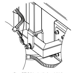
Figure 7.19: Safety wire attachment detail
