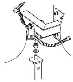
Figure 7.10: M12 Aerotight nut tightening
