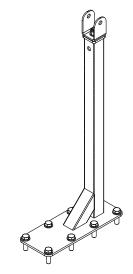
Figure 7.20: AMMB wall/ceiling bracket
