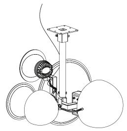
Figure 7.34: Safety wire attachment
