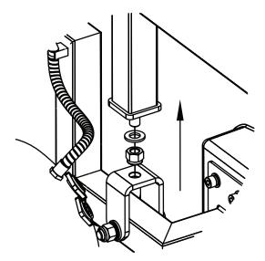
Figure 7.17: Air Motion wall mount detail
