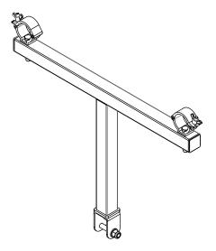
Figure 7.25: AMTB truss mount bracket
