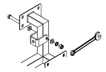
Figure 7.5: M12 x 70 mm bolt insertion
