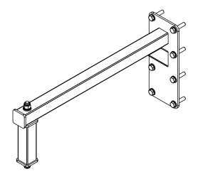
Figure 7.13: AMMB wall/ceiling bracket with extension piece
