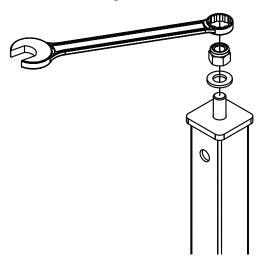
Figure 7.8: M12 Aerotight nut removal
