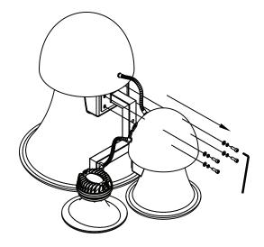
Figure 7.2: M8 socket cap removal
