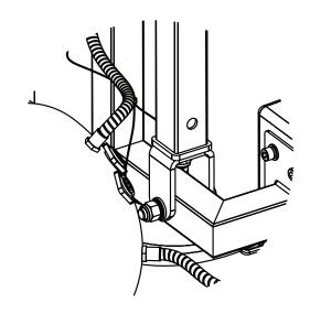
Figure 7.24: Safety wire attachment
