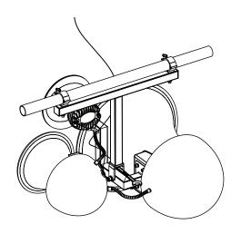
Figure 7.30: Safety wire attachment
