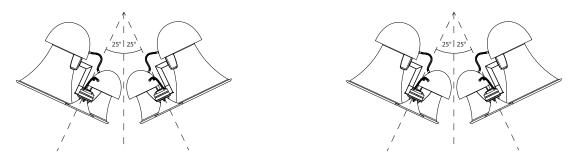
Figure 6.2: Air Motion dual pair arrangement
