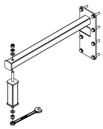
Figure 7.14: Extension piece assembly
