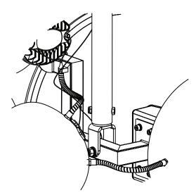
Figure 7.35: Safety wire detail
