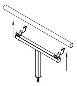
Figure 7.26: Positioning the truss bracket
