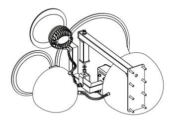
Figure 7.16: Air Motion wall mount
