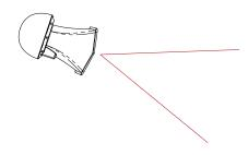
Figure 6.5a: Vertical dispersion (side view)
