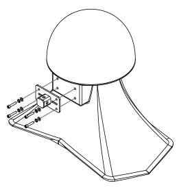
Figure 7.9: Air Series stud mount bracket positioning
