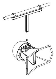
Figure 7.33: Air Vantage truss mount
