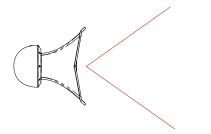
Figure 6.5b: Horizontal dispersion (top view)
