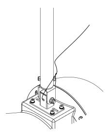
Figure 7.24: Safety wire attachment detail
