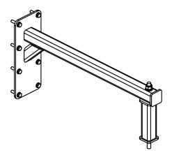
Figure 7.16: WHD wall/ceiling mount with extension piece
