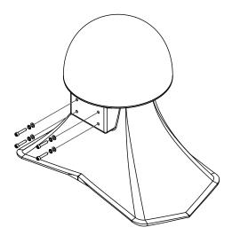
Figure 7.8: M8 socket cap removal
