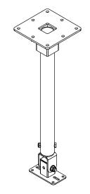
Figure 7.20: Air series ceiling bracket
