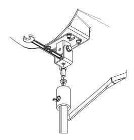
Figure 7.27: Mounting to the U bracket
