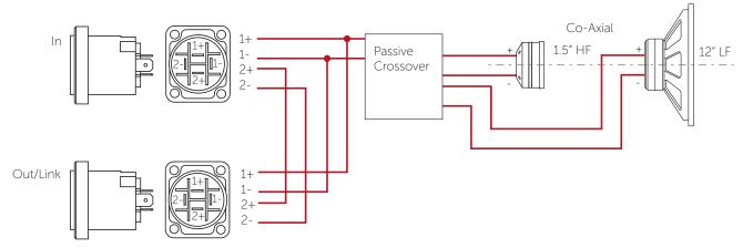
Figure 5.1: Air Vantage wiring diagram
