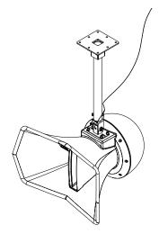
Figure 7.23: Safety wire attachment
