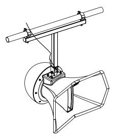
Figure 7.35: Safety wire attachment
