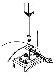
Figure 7.34: Air Vantage truss mount detail
