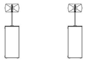
Figure 6.3: Air Vantage bass cabinet mounting
