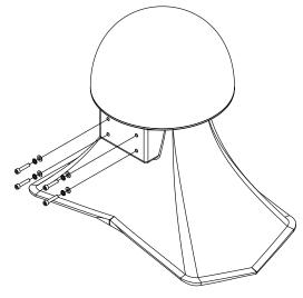
Figure 7.2: M8 socket cap removal
