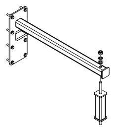
Figure 7.17: WHD wall/ceiling mount with extension piece fixing
