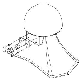
Figure 7.3: Air Series pole mount bracket positioning
