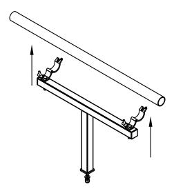
Figure 7.31: Positioning the truss bracket
