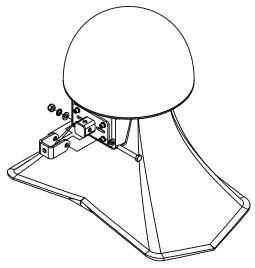
Figure 7.11: Air Series stud mount U bracket fixing
