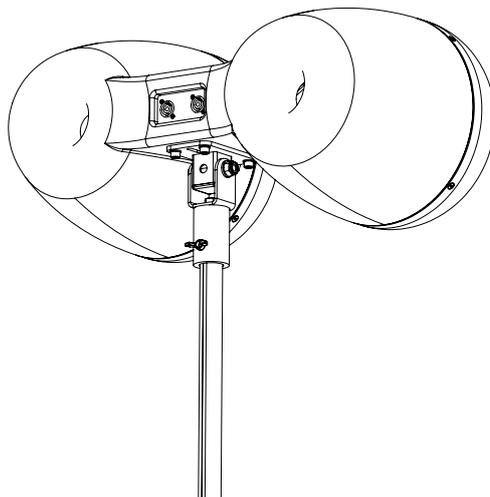
Figure 7.29: Adjusting the loudspeaker position
