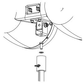
Figure 7.27: Mounting to the U bracket
