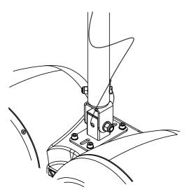
Figure 7.24: Safety wire attachment detail
