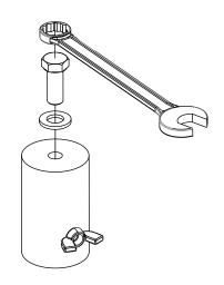
Figure 7.26: Pole mount bracket removal
