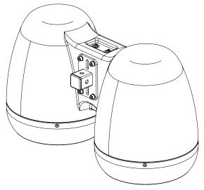
Figure 7.10: Air Series stud mount bracket fixing
