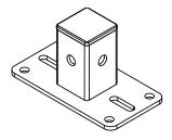
Figure 7.7: Air Series stud mount bracket
