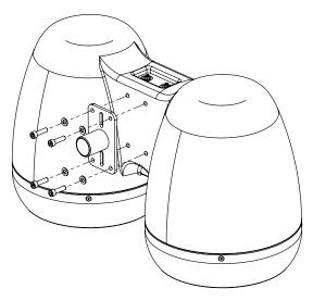
Figure 7.3: Air Series pole mount bracket positioning
