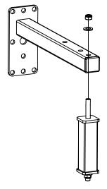
Figure 7.17: WHD wall/ceiling mount with extension piece fixing
