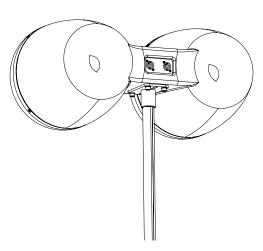
Figure 7.6: Air Series pole mount
