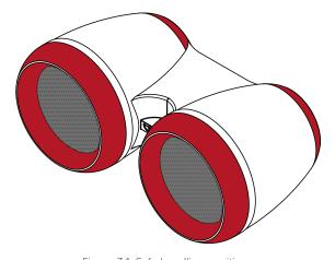
Figure 3.1: Safe handling positions (as indicated in red)
