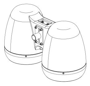
Figure 7.4: Air Series pole mount bracket fixing
