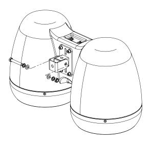
Figure 7.11: Air Series stud mount U bracket fixing
