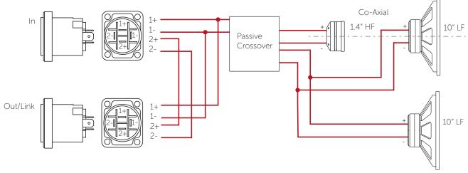
Figure 5.1: Airten V3 wiring diagram
