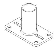
Figure 7.1: Air series pole mount
