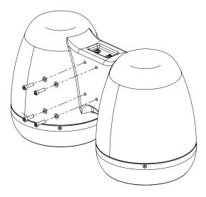
Figure 7.2: M8 socket cap removal
