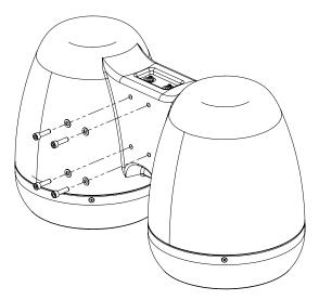
Figure 7.8: M8 socket cap removal
