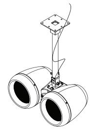
Figure 7.23: Safety wire attachment
