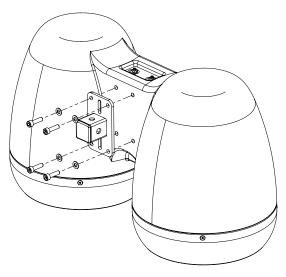
Figure 7.9: Air Series stud mount bracket positioning
