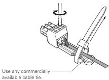
2. Loosen the screws with a flathead screwdriver.
