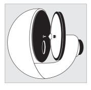
To attach plastic bossed push-on effect wheels, simply push the wheels onto the shaft of the wheel rotator as per the image left.
