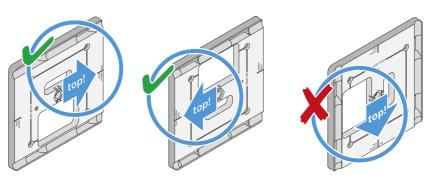
▶ Make sure that the mounting frame is aligned correctly.
