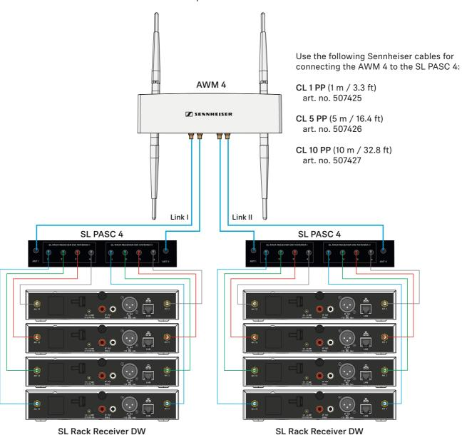
Cables for connecting the SL PASC 4 to the SL Rack Receiver DW are supplied with the SL PASC 4.
