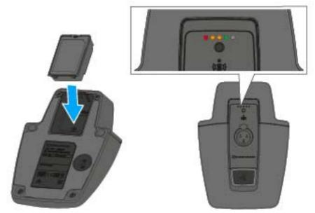
Slide the accupack into the compartment with the correct orientation until the unlock button locks into place.
