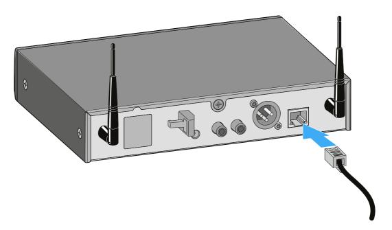
▶ Connect the other end of the network cable to a router or a switch.
