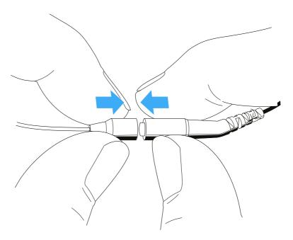
▶ Slide the silicone tube onto the connector.
