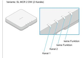
When the LEDs are displaying the status of the entire device and not the individual channels, all four LEDs (SL MCR 4 DW variant) or the first two LEDs (SL MCR 2 DW variant) will light up or flash.
