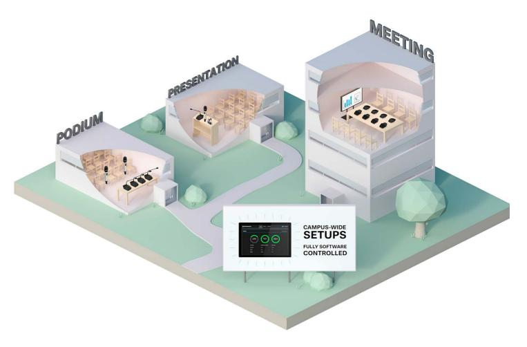
When planning the installation of a wireless audio system, there are some aspects to be considered such as the number and size of the rooms to be equipped or the number of the wireless microphone links you plan to install.
