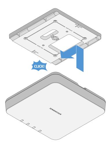
> Insert the receiver into the mounting frame as shown until you hear it click into place.
