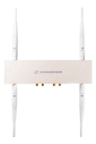
With the AWM 4 antenna wall mount, the antennas can be remote mounted – optimally positioned and nearly invisible – from the receivers (e.g. when the receivers have to be installed invisibly or when the receiver position is not the best antenna position for optimum reception). The AWM 4 can be easily mounted on a microphone stand or permanently installed on a wall.
