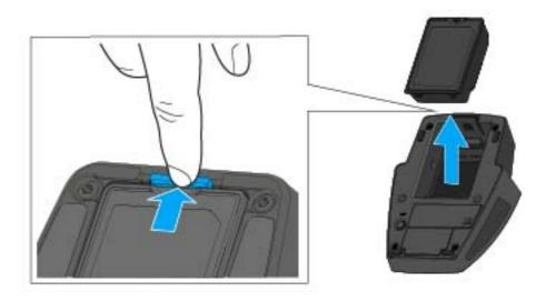
▶ Pull the unlock button away from the accupack and pull the accupack out of the compartment.
