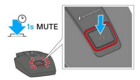
▶ While the table stand is switched on and a goose neck microphone is connected, press the ON/OFF button for 1 second.
