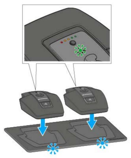
▶ Place the table stand on the CHG 2W charging base in the area marked. If the table stand is positioned correctly on the charging surface, the alignment LED lights up green.
