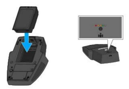
Slide the accupack into the compartment with the correct orientation until the unlock button locks into place.
