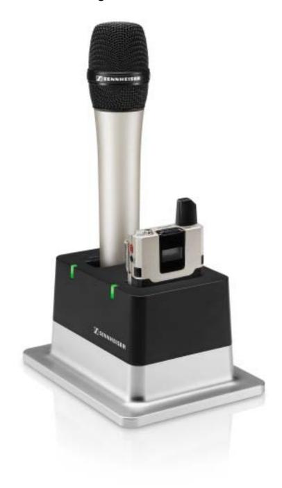
The CHG 2 charger allows you to simultaneously charge up to two transmitters of the SpeechLine Digital Wireless series. A bi-color LED at each charging slot provides information on the current charge status. The charger has universal charging slots for charging both handheld and bodypack transmitters.
