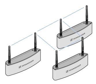
▶ If possible, position the antennas so that there is a direct line of sight (without obstacles) between the transmitters and the antennas.
