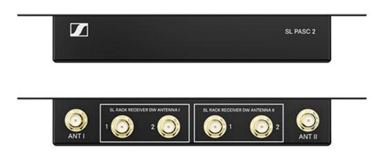
The SL PASC 2 is a passive two-way true diversity antenna splitter/combiner for the SpeechLine Digital Wireless microphone series. It is used to distribute the antenna signals from up to 2 SpeechLine Digital Wireless radio links. In combination with the AWM 2 or AWM 4 remote antennas, the number of required antenna cables is reduced to a minimum. The rack receivers are connected to the SL PASC 2 using the supplied SMA-R cables.
