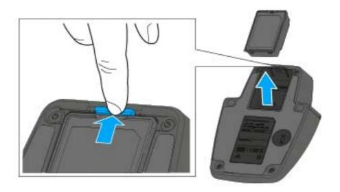
▶ Pull the unlock button away from the accupack and pull the accupack out of the compartment.
