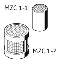
In addition, the large frequency response cap attenuates wind noise by approx. 15 dB and provides an extended protection against the ingress of moisture.
