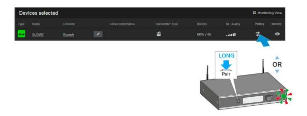
First, **Identify** appears on the display panel of the receiver. The **Pairing** message then appears.
