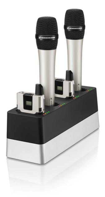
The CHG 4N is a network-compatible charger with four separate charging slots. These ports can be used for the SL Bodypack DW and the SL Handheld DW. The four LEDs on each charging slot indicate the current charging status. The versatile network interface is compatible with IPv4 and IPv6 for seamless integration. The Sennheiser Control Cockpit software can be used to monitor and remotely control the settings and status messages.
