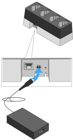
□ Guide the cable through the cable guide at the base of the charger so that the charger is stable once in position.
