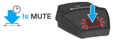
▶ If the boundary microphone is on, press the ON/OFF button for 1 second
