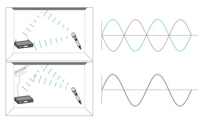
The signal is reflected by the electrically conducting surface. At worst, the blue signal and the red reflected signal are out of phase when they reach the receiver so that the two signals cancel each other out.
