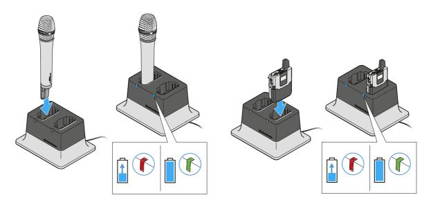
▶ Insert the transmitter with the accupack installed and with the charging contacts facing downwards into the charger.
