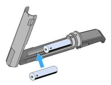
To insert the accupack or the battery compartment:
