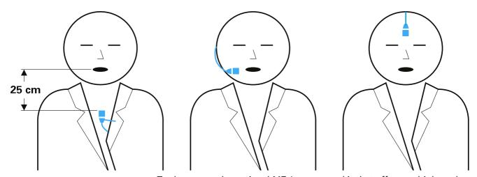
To do so, use the optional MZ 1 accessory kit that offers multiple and secure attachment possibilities. The clips, holders and mounts are suitable for almost any wearing situation and ensure optimum sound quality.
