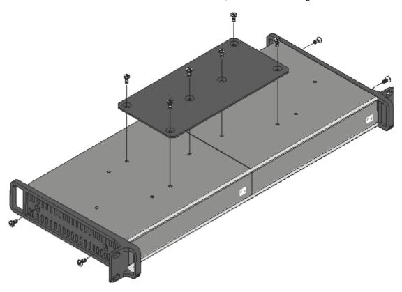
> Screw the unit consisting of the two antenna splitters into a 19" rack.
