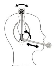
Slide the boom to position the microphone within 13 mm (1/2 inch) of the right corner of your mouth.
