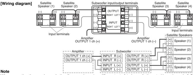
When operating the speaker as in the diagram above (amplifier output of 1 channel), the rated impedance is 8  $\Omega$ .
