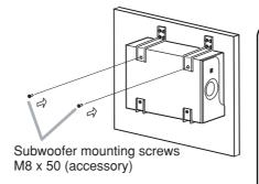
Step 5. Mount 2 subwoofer mounting brackets to the speaker's upper side as well.
