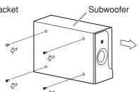
**Step 2.** Remove 4 screws on the subwoofer's side panel.
