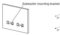
**Step 1.** Mount 2 subwoofer mounting brackets to the wall.
