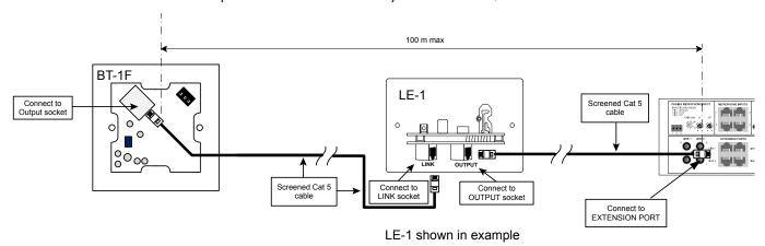
If multiple LE-I/BE-Is are "daisy-chained" to an Extension Port, the BT-IE should be connected to the **LINK** connector of the "last" LE-I/BE-I in the chain. Note that as the BT-IE has no Link connector, it must always be the last module in a chain.
