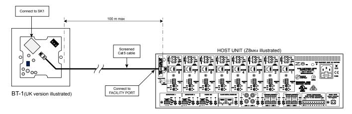
The maximum total Cat 5 cable length should not exceed 100 m. If further modules are being "linked" together (see "Connecting a BT-1F to an LM-2" on page 10), this figure applies to the overall cable run from the host unit to the farthest module in the chain.
