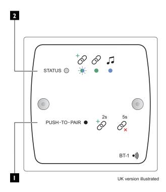
1. **PUSH-TO-PAIR** – recessed push-button accessed through a 2 mm dia. hole. The two "chain" symbols adjacent to the access hole depict the effect of "short" and "long" presses on the button:
