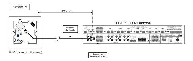
**IMPORTANT:** Note that on the DCMI and DCMIe Digital Control Zone Mixers, the four Extension Ports are alternative input connectors for Line Inputs I to 4. When a BT-IE is connected to an Extension Port, the corresponding pair of Line Input phono connectors must not be connected to a music source device of any kind.
