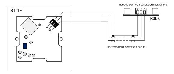
An RL-I/RSL-6 connected to a host unit via a BT-IF in this manner will only operate correctly if the host's Music Control functions have been correctly configured. For details of how to do this, please see the Installation Guide for the host unit.
