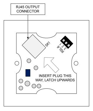
LOCATION OF REAR RJ45 CONNECTOR (Sketch simplified; only primary components shown)
