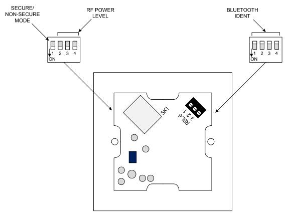
DIP switches shown with factory default settings (Sketch simplified; only primary components shown, BT-1F shown as example)
