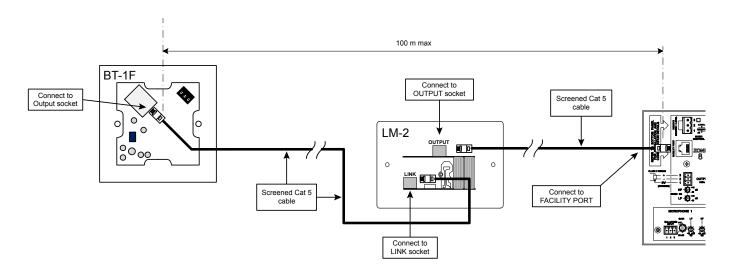
If multiple LM-2s are "daisy-chained" in the Zone, the BT-1F should be connected to the **LINK** connector of the "last" LM-2 in the chain. Note that as the BT-1F has no Link connector, it must always be the last module in a chain.
