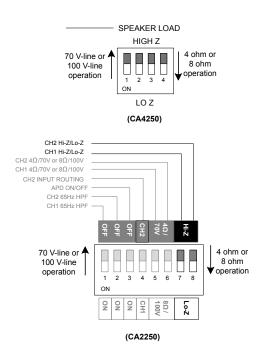
The output mode may be set independently for each channel. Set the switch UP for high impedance (70/100 V-line) operation and DOWN for low impedance operation.
