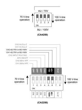
The voltage may be set independently for each channel. Set the switch UP for 70 V line operation and DOWN for 100 V line operation.
