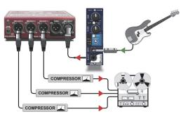
Connect your favorite microphone and compare how it sounds using several preamps to find the best match to suit the vocalist. The Cherry Picker makes it easy and fast. Or, optimize the sound of the bass by comparing compressors. Connect the bass to the JDV-pre instrument preamp and use the Cherry Picker to listen to various compressors.
