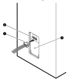
3 Use a flat-bladed screwdriver to turn the input selection switch § on the back of the loudspeaker, and then select the transmission method (100 V / 70 V / 8  $\Omega$ ) and input wattage.
