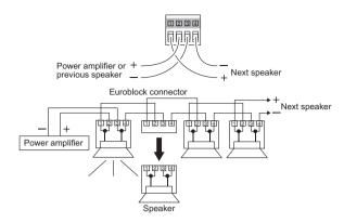
1 Strip away about 7 mm (0.3") of the insulation on the end of the speaker cable, insert the core wire of the speaker cable into each terminal of Euroblock connector 1, and tighten the screw 2 to secure it.
