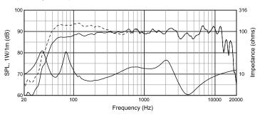
On axis in half-space (2pi, dotted line) and full-space (4pi, solid line) at thru (8 ohm) setting Input Impedance
