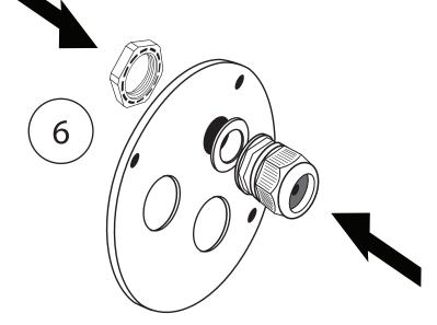
Attach one of the two included Gland Nuts into the open hole on the seal plate as shown above.
