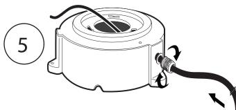
Install the gland nut into the hole as shown above in #6 and feed external wire from outside through the gland nut and up through the center hole in the lower half of the speaker as shown above.
