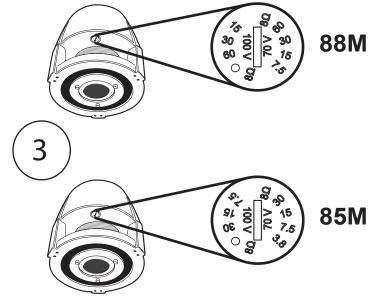
Close-up view of tap setting for the Control 85M and Control 88M. \*\*Adjusting tap setting required before powering up system.
