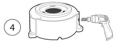
The second gland nut can be installed by drilling a 22 mm (7/8 in, 0.875 in) hole on the side of the bottom half of the enclosure, in one of three recesses on the underside of the enclosure, or other locations as needed, while taking care that the location chosen does not interfere with the locking parts so both halfs of the enclosure will mate and close properly.
