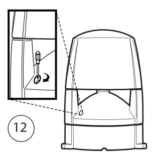
Using included security screwdriver, and making sure you have lined up the security screw with brass nut, turn clockwise so screw will lock top and bottom section together.
