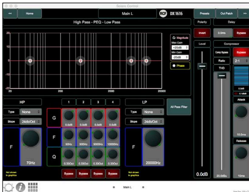
Figure 12: Example of DSP module “Main L”
