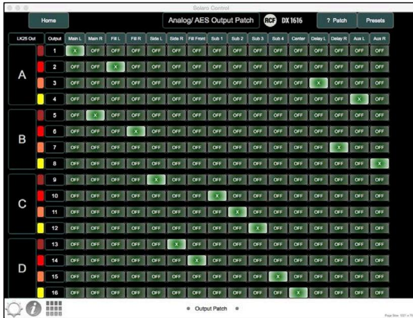
Figure 15: Analog/ AES output patch
