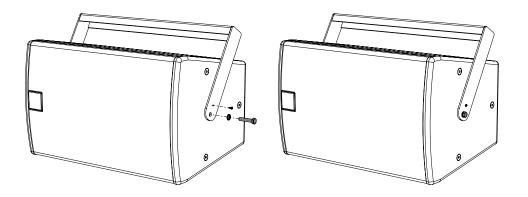
The U brackets A,B,C & D are specifically designed for hanging Cuboid from a ceiling in landscape mode. Fixing the U bracket is a simple process:
