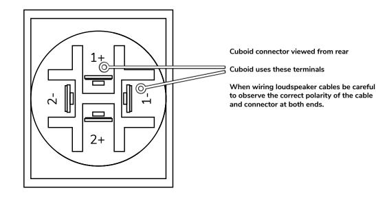
All Cuboid loudspeakers are fitted with two standard NL4 type connectors. These have two pairs of terminals.
