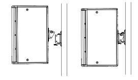
Lift loudspeaker into position making sure that the two halves of Wall Bracket line up – the adjustable bolt sits into the two 'U shaped' cups in the wall section of the bracket
