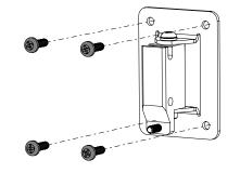
Once loudspeaker position has been decided, affix wall section of Wall Bracket (A,B or C depending on Cuboid model) securely to a suitable wall mounting point
