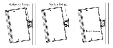
Once the loudspeaker is in position and you are happy with the angle adjustments, tighten all fixings as shown to lock the cabinet in place.
