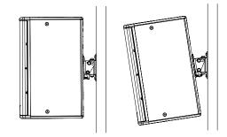
Secure the assembly with the fixed bolt in the lower hole in the bracket – this provides the pivot for angling the loudspeaker. Adjust the grub screw to fix the down-tilt angle
