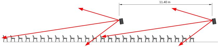
Because of this level drop over distance, in larger rooms it's well worth considering additional loudspeakers to counter this effect, maintaining volume and intelligibility. In this case, it is important that the second row of loudspeakers down the room are delayed to match the arrival of the sound from the first pair of speakers, as shown above.
