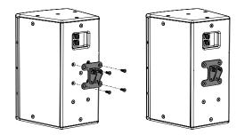
Position loudspeaker cabinet section of Wall Bracket over the four M8 mounting points and secure with the four bolts from the back of the cabinet
