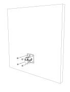
The orientation of the loudspeaker fixing plate can be pre-set and tightened using the supplied 4mm hex wrench. Use the supplied 3mm hex wrench to fix the loudspeaker to the bracket.
