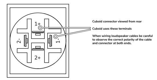
Cuboid 8, 10, 12 and 15 are fitted with two standard NL4 type connectors. These have two pairs of terminals. Cuboid uses only pins 1+ and 1-. These are linked across the two connectors, providing a useful link to a second loudspeaker of the same model. No more than two Cuboids should be connected to a single amplifier channel. 2+ and 2- are not connected and are not linked through. For connection, we recommend using a flexible cable with a minimum cross-sectional area of 1.5mm<sup>2</sup>
