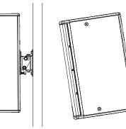
Once the loudspeaker is in position and you are happy with the angle adjustments, tighten all fixings as shown to lock the cabinet in place.
