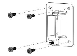
Position loudspeaker cabinet section of wall bracket over the four M8 mounting points and secure with the four bolts from the back of the cabinet. Remove M8 fixing bolts from the rear of the loudspeaker cabinet.
