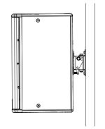
Secure the assembly with the fixed bolt in the lower hole in the bracket – this provides the pivot for angling the loudspeaker. Adjust the grub screw to fix the down-tilt angle.
