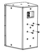
Optional wall bracket mounting positions enable greater down-tilt, using the lower four M8 bolt position, or the loudspeaker can be mounted in landscape mode by rotating the bracket as shown: he loudspeaker to the bracket.
