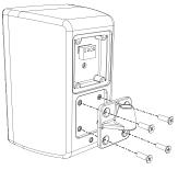
Attach the loudspeaker and bracket assembly to the wall mount and tighten in the desired orientation.
