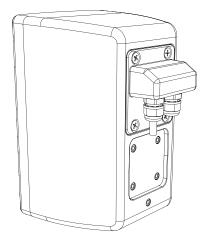
Finally, tighten the cable gland onto the cable(s) to provide a good seal. If only one gland is used, tighten the second as far as you can.
