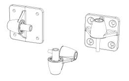
It is critical that the structure to which Cuboid is to be mounted is suitable for taking the weight of the loudspeaker/bracket assembly. It is highly recommended that a secondary safety fixing be fitted. The wall bracket is fixed to the mounting position by 4 screws as shown.
