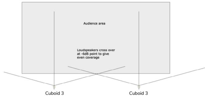
2 x Cuboid 3 positioned to overlap horizontal coverage
