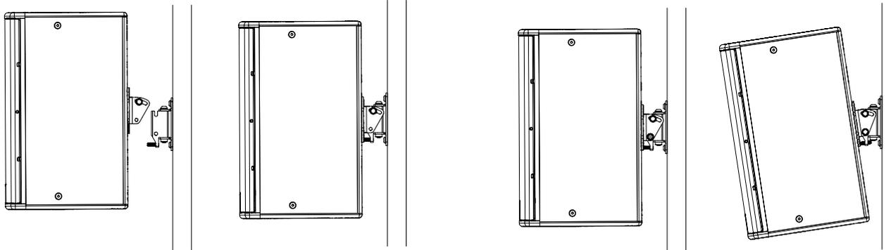
Once the loudspeaker is in position and you are happy with the angle adjustments, tighten all fixings as shown to lock the cabinet in place.
