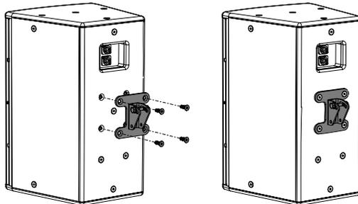
Remove M8 fixing bolts from the rear of the loudspeaker cabinet.
