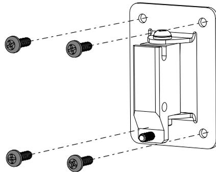
Position loudspeaker cabinet section of wall bracket over the four M8 mounting points and secure with the four bolts from the back of the cabinet.
