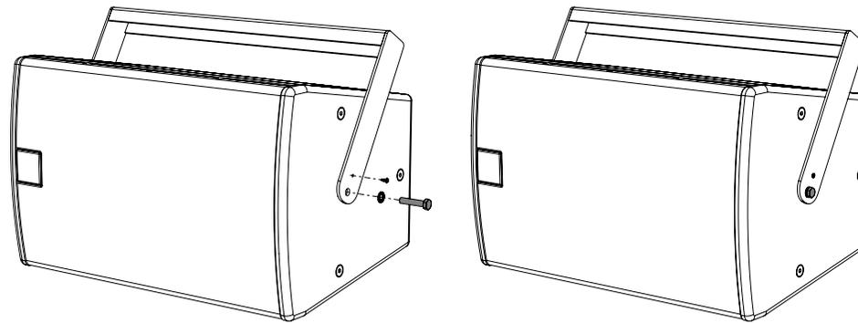
The U brackets A, B, C and D are specifically designed for hanging Cuboid from a ceiling in landscape mode. Fixing the U bracket is a simple process:
