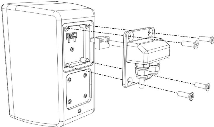
Where present, make sure you have the correct tapping selected from the rotary control beneath the input connector. Then push the cable mounted connector into the speaker, and slide the cover over the cable until it fits against the recess in the back of the speaker.
