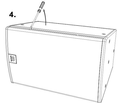
Repeat this process for the remaining gaps in the grille to ease it out of the slot all the way up one side of the cabinet; when you get to the final gap the grille should pop out and away from the front of the cabinet.
