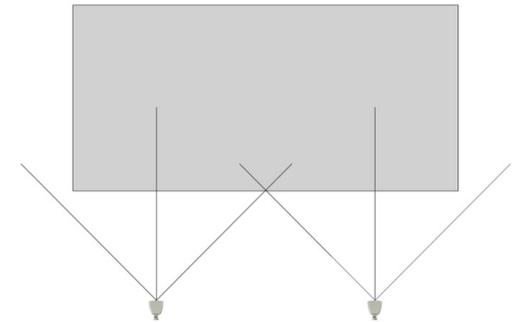
For Cuboid 8 and upwards, the horizontal dispersion is narrower, and the loudspeakers will necessarily be placed closer together, or further away from the listeners for seamless horizontal coverage.
