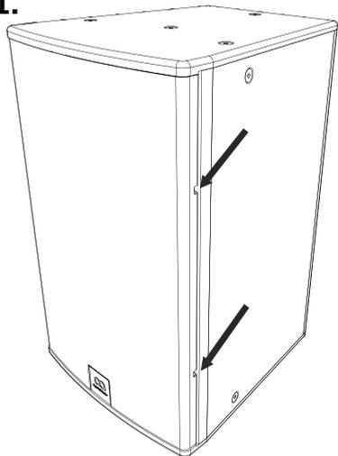
Insert the screwdriver blade into one of the gaps - either at the top or bottom of the cabinet.
