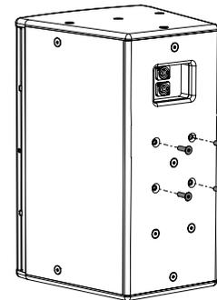
Optional wall bracket mounting positions enable greater down-tilt, using the lower four M8 bolt position, or the loudspeaker can be mounted in landscape mode by rotating the bracket as shown: the loudspeaker to the bracket.
