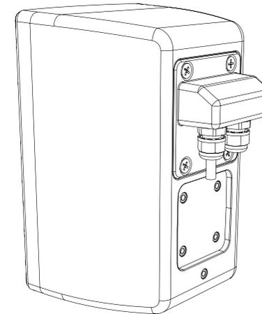
Finally, tighten the cable gland onto the cable(s) to provide a good seal. If only one gland is used, tighten the second as far as you can.
