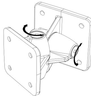
Once the wall mounting part is fixed, attach the loudspeaker part of the bracket to the mounting points on the back of Cuboid 3, 3TX, 5, 5TX, 6 and 6TX.
