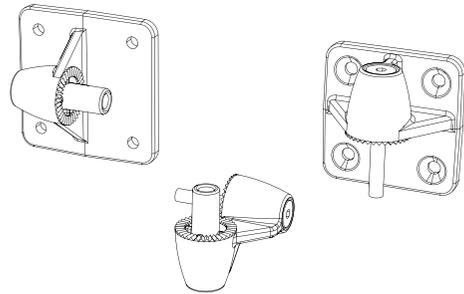
It is critical that the structure to which Cuboid is to be mounted is suitable for taking the weight of the loudspeaker/bracket assembly. It is highly recommended that a secondary safety fixing be fitted.
