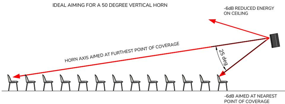
Loudspeaker axis aimed at the furthest point of the desired coverage area
