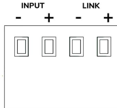
Cuboid 3, 3TX, 5, 5TX, 6 and 6TX loudspeakers are fitted with four pin push-in euroblock connectors.
