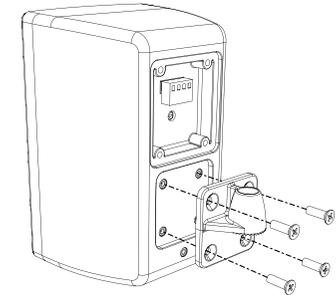
Attach the loudspeaker and bracket assembly to the wall mount and tighten in the desired orientation.
