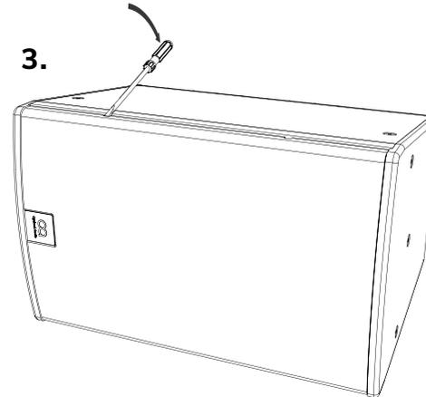
Now lift the handle up; this will ease the grille forward slightly to prevent the return on the grille dropping straight back into the slot:
