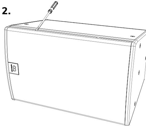
Gently push the handle down. This will ease the grille out of the slot, it may have bitten into the paint surface, so you just need to make sure it is free to be lifted clear.
