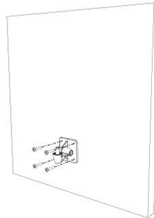
The orientation of the loudspeaker fixing plate can be pre-set and tightened using the supplied 4mm hex wrench. Use the supplied 3mm hex wrench to fix the loudspeaker to the bracket.
