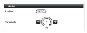
The limiter is active by default; it may be disabled by setting the Enabled switch to Off.
