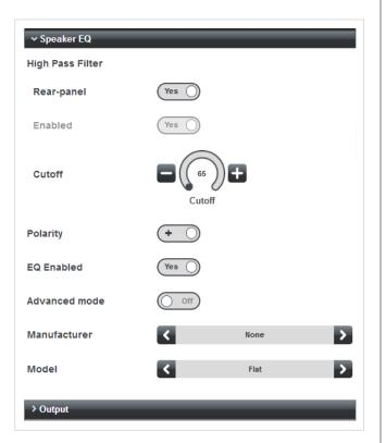
In this mode, it is possible to select a specific loudspeaker EQ preset from a set that has previously been installed. Installation of loudspeaker presets is via a firmware update.
