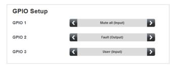
The port has three separate pins (GPIO 1, GPIO 2 and GPIO 3), each which may be configured in one of four ways – two input options and two output options. See "The GPIO Port" on page 50 for electrical and connection details of the GPIO port.
