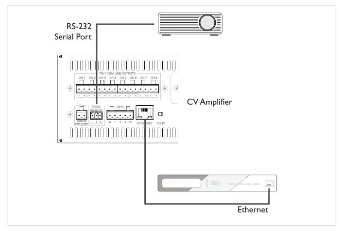
This function uses the amplifier's Bridge Port, whose address has the default value of 4998. If the controlling device is only able to support remote ports in a certain address range (i.e., not including 4998), the port address can be changed on the **Network Configuration** page of the browser interface (select **Config > Networking**).
