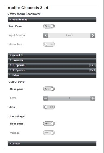
Note that the revised status of Channels 3 and 4 - 2 Way Mono Crossover - is confirmed at the top of the Audio page. The page is now divided into seven tabs: Input Routing, Room EQ, Crossover, HF Speaker, LF Speaker, Output and Limiter. The facilities on the Input Routing, Room EQ, Output and Limiter tabs are identical to those on a standard mono or stereo channel; the Speaker EQ tab is replaced by three tabs related to bi-amped operation.
