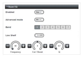
The Q control adjusts the bandwidth of the peaking filter over a range of 0.1 (broad) to 20 (narrow), with a default value of 0.7.
