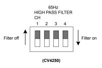
The factory default filter frequency is 65 Hz, which should be satisfactory for many installations; however the frequency can be adjusted over the full audio bandwidth from the web browser pages. Note also that the DIP switch may be disabled, on a per-channel basis, from the web browser pages.
