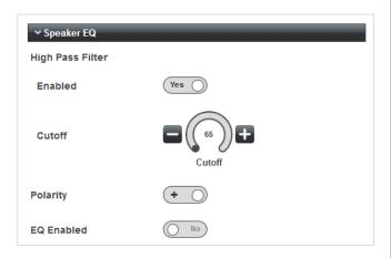
The high-pass filter is out of circuit by default, with Enabled set to No. This ensures the auxiliary channel has its full frequency response. The filter may be inserted by setting Enabled to Yes.
