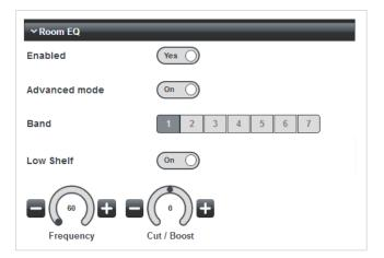
The Room EQ is now reconfigured as a seven band parametric equaliser, with peak/shelf switching on the highest and lowest bands. The Band buttons assign the rotary controls to each frequency band in turn: all bands have the same frequency range of 20 Hz to 20 kHz, adjusted by the Frequency control. However the seven default centre frequencies are 60 Hz, 250 Hz, 1 kHz, 2 kHz, 4 kHz, 8 kHz and 16 kHz, which will be suitable for most installations. The Cut / Boost control has a range of +/-12 dB.
