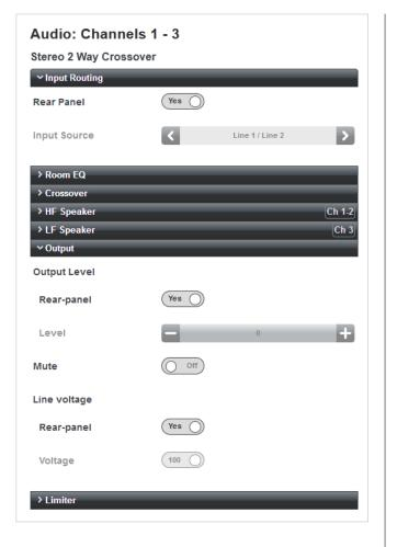
The status of the three channels is confirmed at the top of the page. The page has the same seven tabs as the 2-Way Mono Crossover Audio page. Note however, that the HF Speaker tab is now annotated Ch 1-2 and the LF Speaker tab Ch 3, indicating that (in this example), these are how the channels are deployed.
