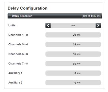
Delay is implemented by entering the delay time in each field as required.
