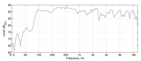
Frequency response (Anechoic measurement)
