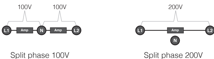
Figure 6:5: Two phase split-phase configuration
