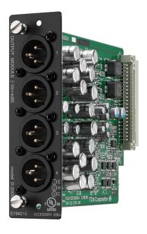
The D-2000DA1 Line Output Module is designed for use with the D-2008SP Digital Mixing Processor Unit and features high quality sound. The output level of each output terminal can be independently set to either +4 dB or -10 dB and its output mode independently set to either balanced or unbalanced type by the built-in DIP switch. It employs XLR type connectors.
