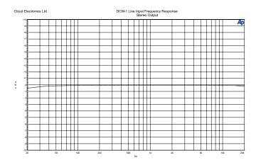
DCMI/DCMIe Line Input Frequency Response Stereo Output
