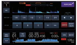
When in slip mode, [SLIP] on the screen bottom left lights up in blue.
