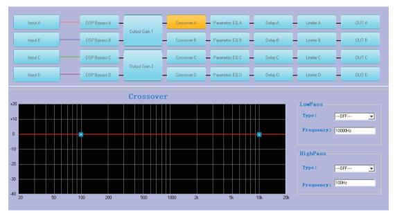
Crossover-Click the image to change the high and low frequency (20Hz-20KHz).
