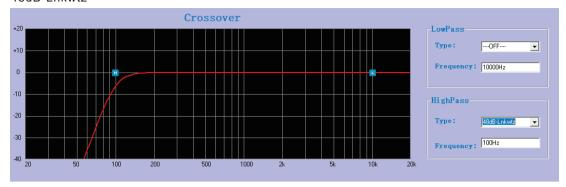
Frequency-Input high pass filter frequency (20Hz~20kHz)
