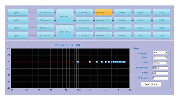
Parametric EQ- the type, frequency, gain and Q value of each segment are settable.
