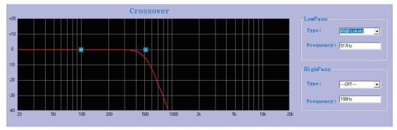
Frequency-Input low pass filter frequency (20Hz~20kHz)
