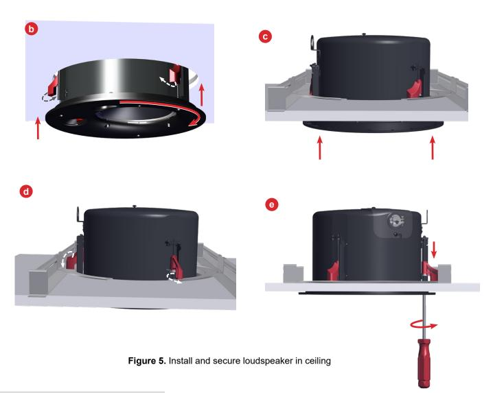
**IMPORTANT:** For closed ceiling applications all connections (wiring and safety cable) must be made with the input cover installed before inserting the unit in the ceiling.
