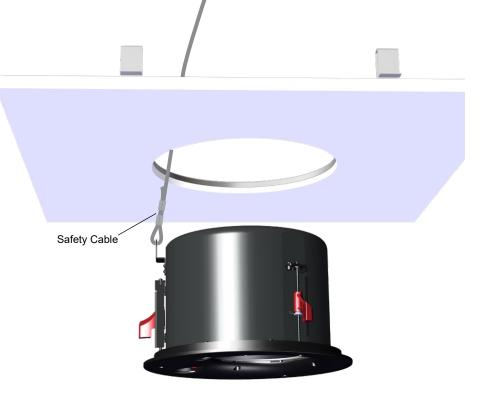
Figure 4. Adjust clamp height and attach safety cable\*
