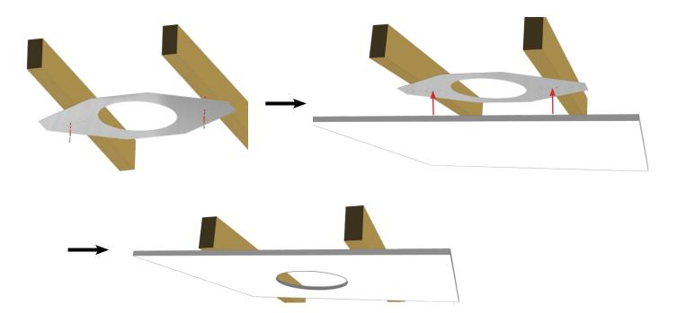
Figure 8. Install bracket and drywall or sheet rock
