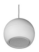
The Apart EN-SPH5T16-W is a compact 5.25" sphere loudspeaker with ABS housing (Ul94 HB) (RAL 9010 equivalent), equipped with a high efficiency full range speaker and a multi tap 100 volt transformer, all certified according EN 54-24.
