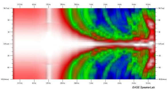
Figure 2: Vertical Directivity Map of One ENTASYS Full-Range Column at 50 meters
