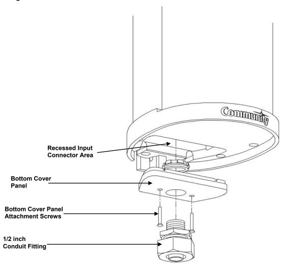
Figure 22: ENTASYS Bottom Cover Panel with Conduit Knock-Out
