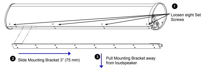
Figure 4: ENTASYS Mounting Bracket Removal
