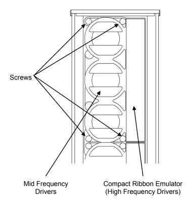
Each of the mid/high frequency modules are attached to the baffle with four, M4 screws. These screw into taped holes in the aluminum baffle. There are no nuts to have to hold or catch inside the enclosure. Shorter screws are used with some of the smaller spacers. These will need to be replaced with the included longer 60mm screws when the larger 34.2 mm spacer is used.
