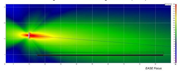
Figure 26: One Full-Range Column (1 kHz)
