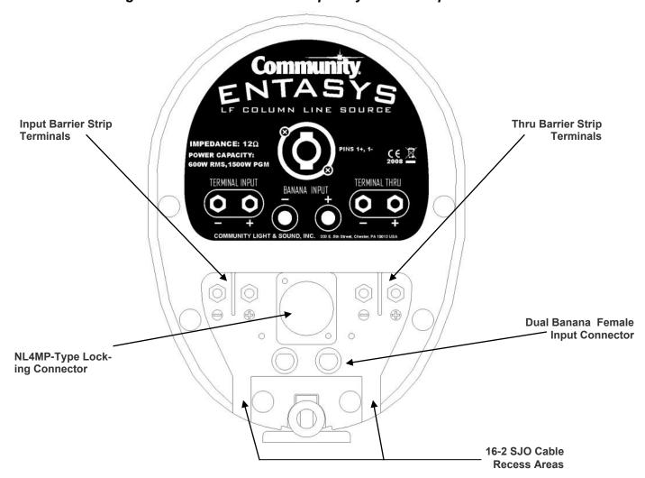
Figure 20: ENTASYS Low Frequency Column Input Panel
