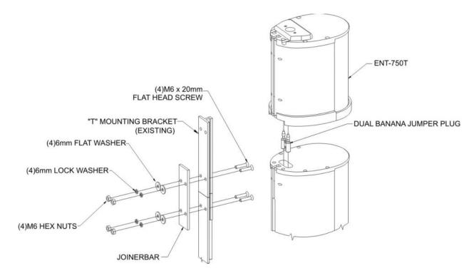
Figure 17: Transformer Mounting On Top of Array
