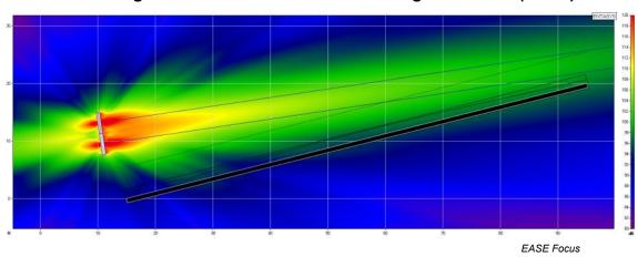
Figure 27: Two ENTASYS Full-Range Columns (1 kHz)
