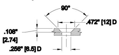
Figure 5: Countersink Detail
