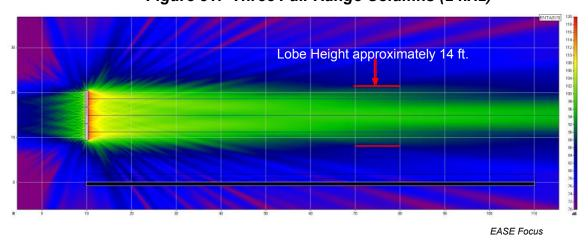
Figure 32: Six Full-Range Columns (2 kHz)
