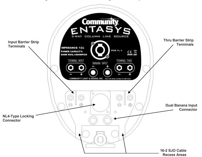
Figure 19: ENTASYS Full-Range Column Input Panel
