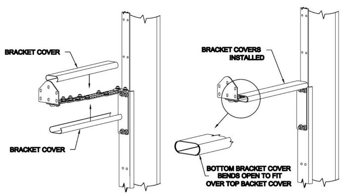
Figure 13: Pan-Tilt Bracket - Cover Assembly
