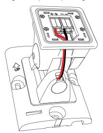
Figure 2. Wire path to wire the ClickMount Bracket (single wire shown)
