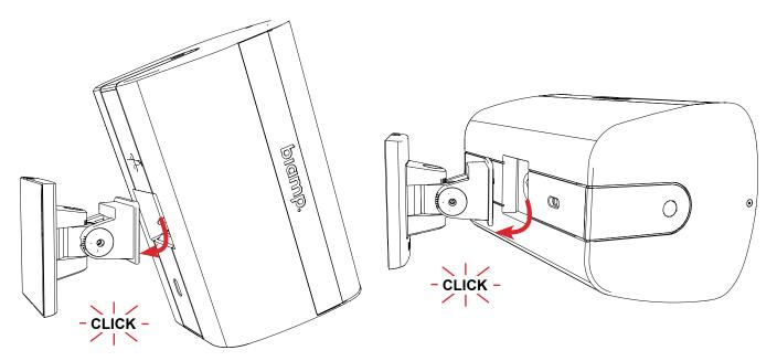
Figure 5. Rotate and press the loudspeakers on the ClickMount bracket
