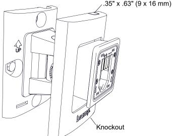
**Figure 3.** Before loudspeaker is attached fit the cover plate on the bracket and press into place
