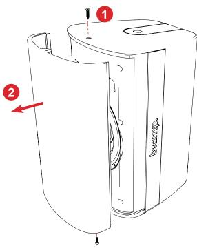
**Figure 19.** After removing the screws, carefully pry off the grille
