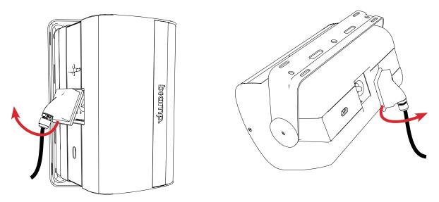
**Figure 15b.** Pull the ClickPlug away from the latch side. Do **NOT** use a tool to remove it as you will mar and/or deform the plastic.
