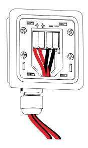
**Figure 9b.** ClickPlug wired with 2 pairs for daisy-chained applications
