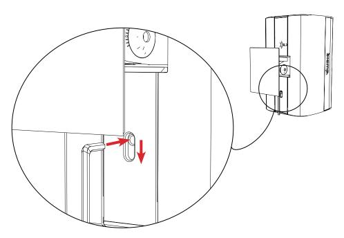
Figure 8a. Insert hex wrench into hole and pull down to release latch
