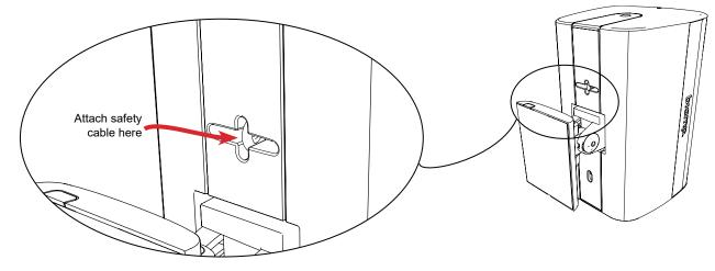
Figure 6. Attach safety cable
