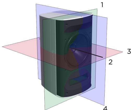
1. Reference Plane (green) is coincident with the front of the LF mounting ring
