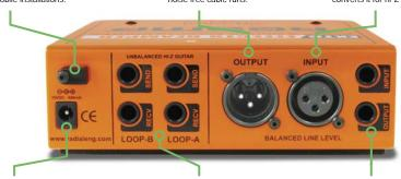
15VDC POWER connection for the external 400mA power supply.
