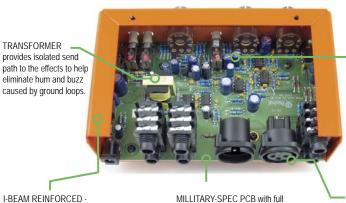
I-BEAM REINFORCED -Enclosure makes it impossible to torquet the PC board & eliminates cold solder joints.
