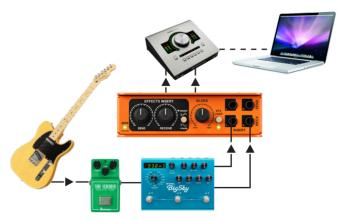
Using the EXTC Stereo for direct recording
