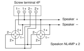
Two Subwoofer Systems can be operated in parallel by connecting them in a cascade configuration as shown below.
