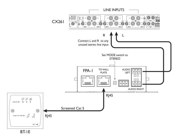
The audio connection between the FPA-I and the CX26I line input is most easily achieved with a pre-made twin phono-phono cable, with the connectors at one end cut off. This can then be connected to the left and right audio outputs of the FPA-I, using the mating connectors provided.
