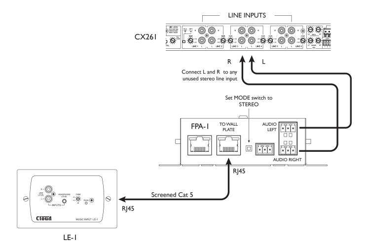
The audio connection between the FPA-I and the CX26I line input is most easily achieved with a pre-made twin phono-phono cable, with the connectors at one end cut off. This can then be connected to the left and right audio outputs of the FPA-I, using the mating connectors provided.
