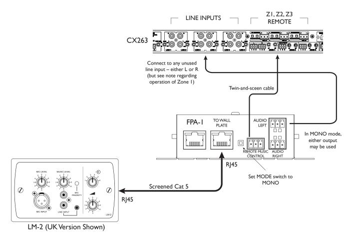
As in Example I, the audio connection to the host unit is most easily made by cutting off the connector(s) from one end of a pre-made phono-phono cable. Wire pins I (screen) and 3 (hot) only at the FPA-I end.
