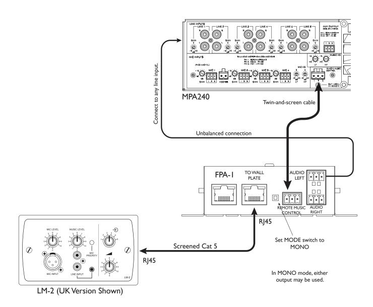
The MPA240 has unbalanced inputs, so a phono cable with one end cut off may be used to connect the audio outputs of the FPA-I to the amplifier. As in Example I, wire pins I (screen) and 3 (hot) only - do not connect pin 2 (cold).
