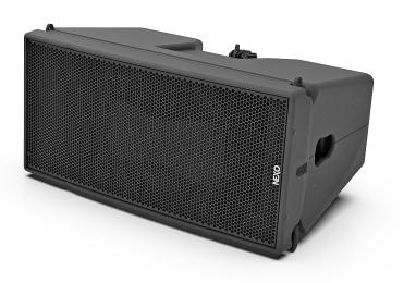
Line array element, 2 way passive or active, with 12" LF and 3" voice coil / 1.4" throat HF.
