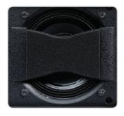
A Directivity Phase Device (DPD) on each cone driver extends the upper frequency limit for file source coupling between adjacent speakers. 6.5" drivers coherently couple as if there were twice as many 3.25" cones mounted at half the physical distance.
