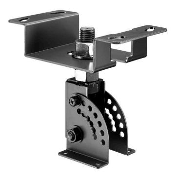
The HY-CW1B is designed to be used exclusively to mount the HX-5 series speaker system to a ceiling. The speaker can be rotated 360° horizontally. It can also be tilted vertically up to 82.5° when suspended horizontally, and depending on the speaker directivity mode, up to 67.5° (for 60° mode) or 75° (for 15°, 30° or 45° mode) when suspended vertically. This bracket is designed for indoor use.
