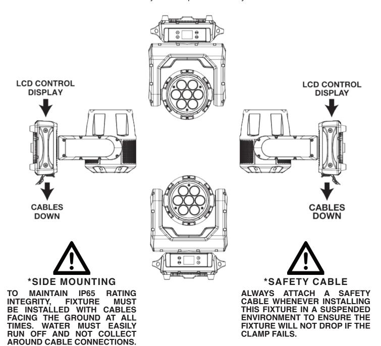
The Hydro Wash X7 is fully operational in three different mounting positions, hanging upside-down, mounted sideways on trussing, or set on a flat level surface. Always use and install a safety cable as a safety measure to prevent accidental damage and/or injury in the event the clamp fails. Never use the carrying handles for secondary attachment.
