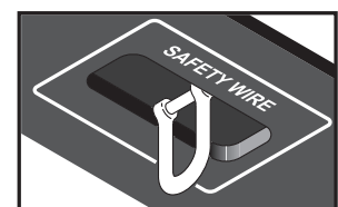
Figure 4: Safety wire attachment point
