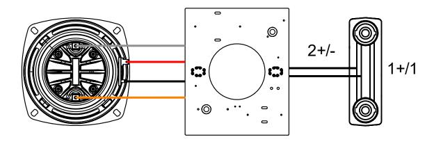
→ ID14i is supplied with a fixed cable (HO7ZZ-F), 2x 0.75mm2 section, length 2m, outside diameter 6.1mm ± 1mm.
