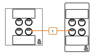
1 Illuminated Buttons – Available functions include Level Up/Down, Mute, Source Selector, External & IP Control, Scene / Preset Select, Room Control.
