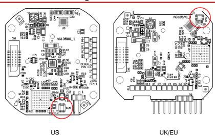
Switch 5 on the main PCB board lets you reset the network settings to factory default. To reset, press the switch for 10s whilst applying power to the unit.
