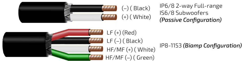
Figure 1b. Standard wiring
