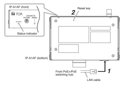
**Step 1.** Connect the speaker to the PoE+ or PoE switching hub using a LAN cable. The speaker will be started.
