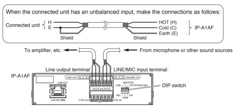
Set the DIP switch according to the audio device to be connected.
