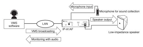
**Tip**Set the local broadcasting settings "OFF." If it is "ON," the microphone input sound will be output to the speaker.
