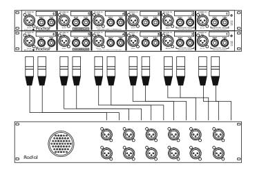
This top figure shows the JD6 with a simple XLR breakout panel called the JD6-X6. This comes standard with 3 feet and 6 feet extensions allowing the breakout panel to be mounted on the back or the front of the keyboard rack.
