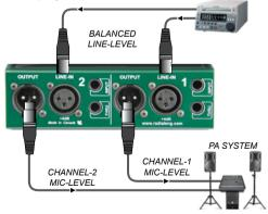
Occasionally you may be confronted with a super powerful source that could overload and saturate the transformers inside the Duplex. This could, for instance, be the output signal from a DJ mixer. If this scenario presents itself, depressing the -15dB PAD switch reduces the input sensitivity and cleans up the signal. If you hear distortion, set the PAD switch to it's inward position. You may have to increase the input level at the mixing desk to compensate.
