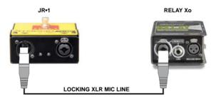
Another advantage is that XLR cables can be dasiy-chained together to make a longer cable. This means you won't have to depend on a specific custom built cable to connect your remote device.
