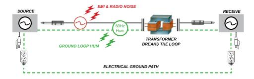
The image above shows an audio source and a destination with a common electrical ground. As the audio also has a ground, these combine to create a ground loop. The transformer and ground lift work together to eliminate the ground loop and potential noise.
