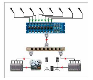
Using the LX8 to feed two different audio systems Running audio around various environments such as large venues, multi-function rooms or broadcast facilities can often lead to noise polluting the audio system. The LX8 eliminates noise problems due to ground loops.
